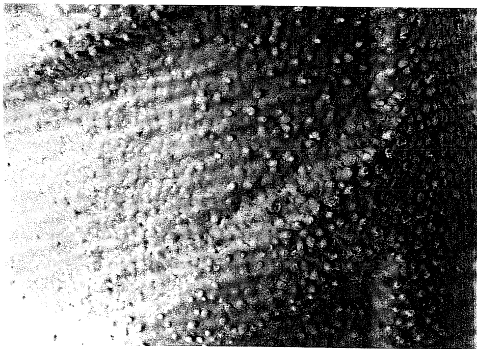
Photo 5.39. Close-up picture showing pin-hole corrosion on the ECR with abnormally rough surface after immersion in 3.5% NaCl solution for 200 days.
