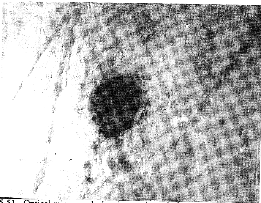
Photo 5.51. Optical micrograph showing a micro pin-hole on epoxy coating with the exposed iron substrate corroded. (x200)
