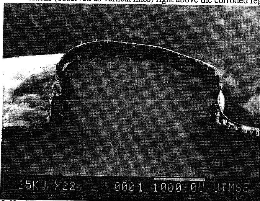
Photo 5.63. SEM micrograph of the ribbed area of a unpatched ECR specimen showing abnormally thin coating on the right hand side of the rib, and corrosion along with coating break due to pin-holes on the left hand side of the rib.
