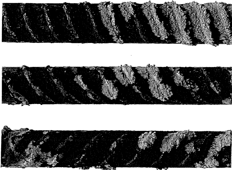
Photo 5.13. Photograph showing typical appearance of uncoated reinforcing steel bars after 105 days of immersion in 3.5% NaCl solution.
